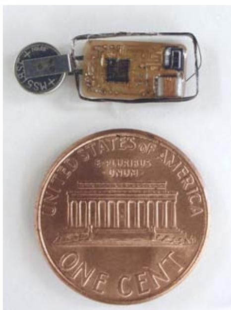
The unpackaged wireless pressure monitor prototype is shown to demonstrate the size of the device and the on-board circuitry that was designed to reduce power consumption and increase efficiency.
