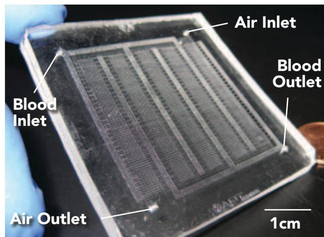
A photograph of the artificial lung showing blood and air inlets and outlets and the microfluidic channels comprising the device. A penny is shown in the background for scale. The artificial lung contains blood channels that are similar in size to those in the natural lung.
