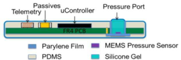
Diagram of the packaged pressure telemetry device.
