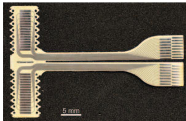
32-contact, microfabricated peripheral nerve cuff for electrical stimulation. The electrode contacts are on the left side of the photograph, while the connection pads are staggered on the right.
