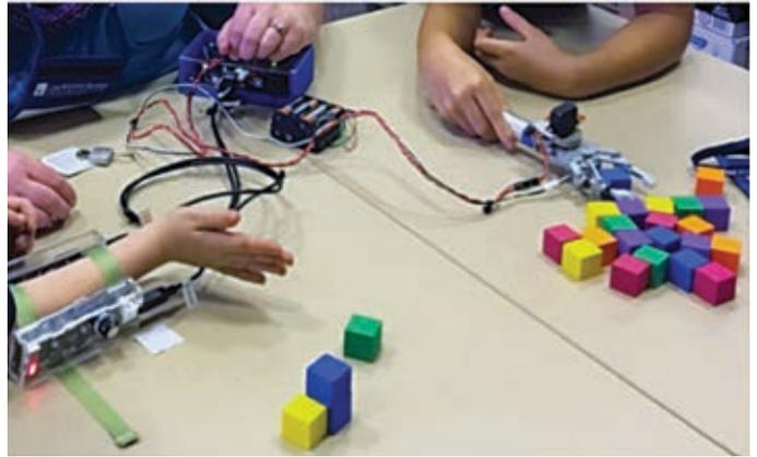
Picking up blocks using the EMG-powered robotic claw
