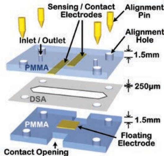
Fabrication drawing of the ClotChip sensor
