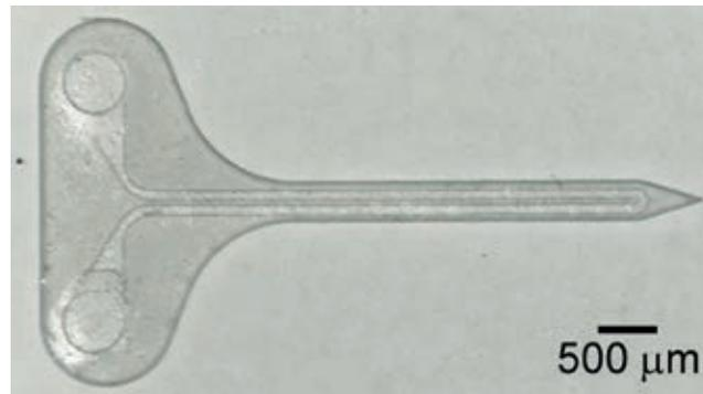
Nanocomposite-based probe with a micromolded, microfluidic channel running through it
