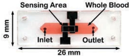
The ClotChip sensor (test strip)
