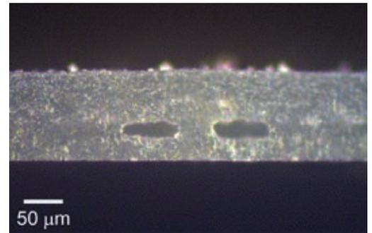
A slice through the microfluidic probe
