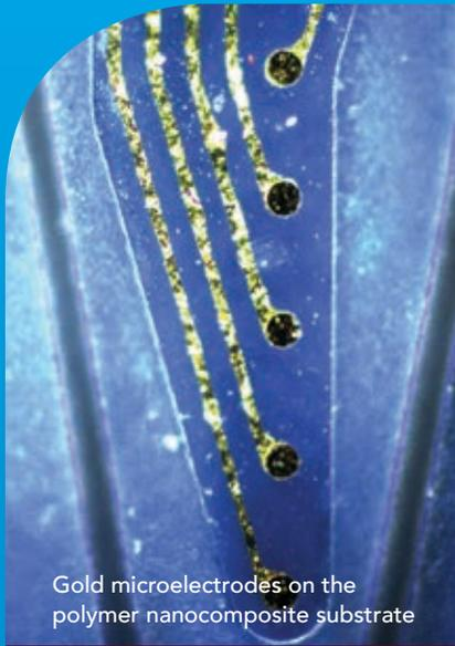
Gold microelectrodes on the polymer nanocomposite substrate
