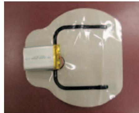
*Working prototype of the Modular Stimulation System for transcutaneous electrotherapy.*
