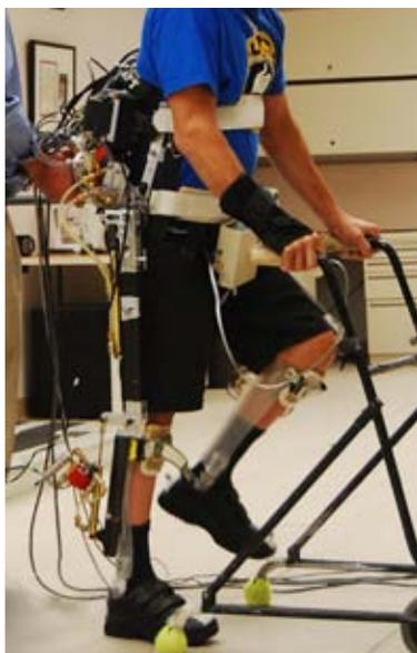
We developed a first generation prototype neuromechanical gait assist system that combined electrical stimulation to the paralyzed lower extremity muscles with a controllable hydraulic exoskeleton for standing, walking, and stair climbing after paralysis. The system consisted of computer controlled knee and hip mechanisms that allowed the lower extremity joints to either move independently, lock to rest the muscles, or couple one motion to another. The system improved walking
